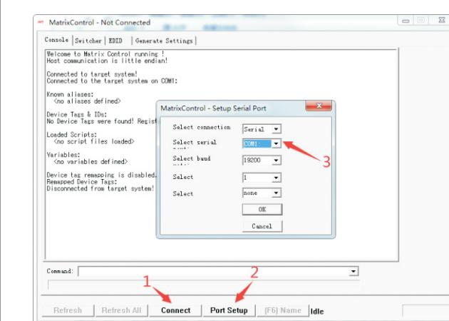
After opening the software, you need to select the corresponding COM to use RS-232 control normally.
